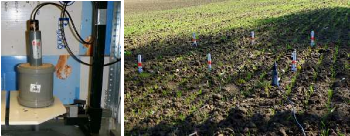
Figure 1: Theta Probe ML2x installed in the sample in laboratory (left) and soil moisture sensors installed in the field – six TMS3 sensors and one Theta Probe ML2x (right).
