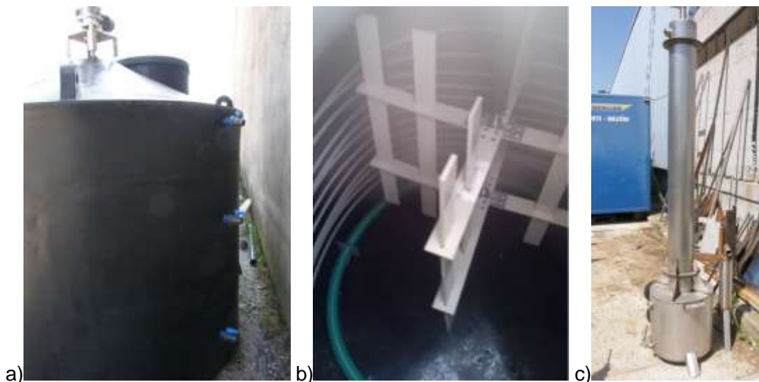
Figure 2: Photographic representation of (a) the compact anaerobic digester showing the sampling ports and the motor, (b) the digester paddle mixing system and the heat exchanger and (c) the biogas scrubber.
