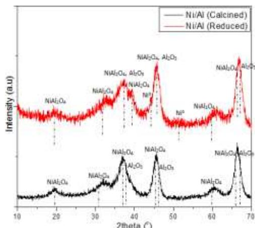
**Figure 1:** XRD patterns of calcined and reduced (at 800°C) Ni/Al catalysts
