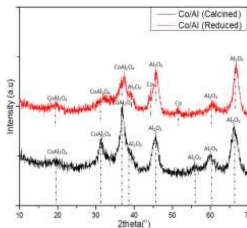
**Figure 2:** XRD patterns of calcined and reduced (at 800°C) Co/Al catalysts
