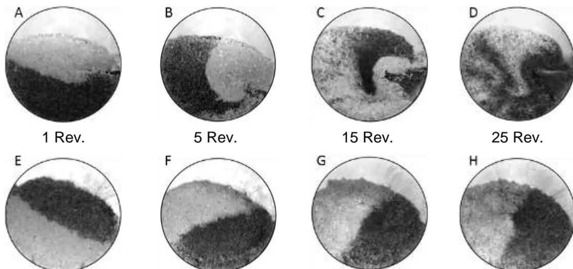
**Figure 1:** Comparison of the radial mixing progress for substrate 1 (A-D, with baffle) and substrate 2 (E-H, without baffle) at 1, 5, 15 and 25 rev. of the RDF (fill level: 0.80).
