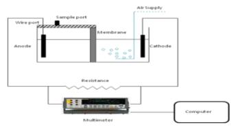
Figure 2: Schematic representation of MFC set-up
