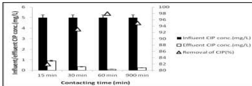
**Figure 7:** Effect of irradiation time on the yields of constant CIP concentration(5 mg/L), at a constant nano GO/M concentration (0.5 g/L), at a pH of 6.5 and at 21°C
