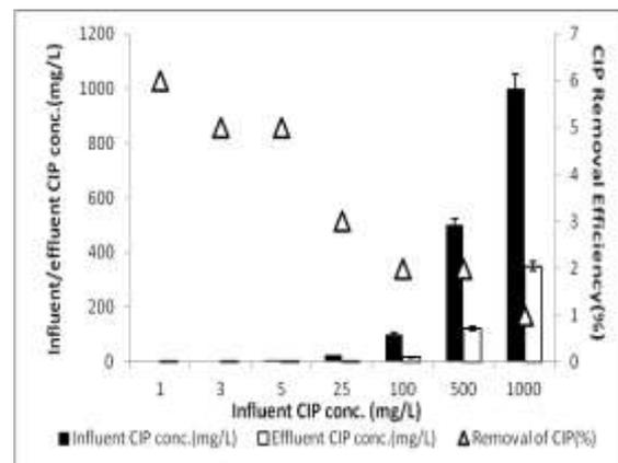
**Figure 1b:** Effect of increasing CIP concentration on the yields of CIP removal at a nano-GO/M concentration of 2 g/L at pH=6.5, at 21°C and 30 min contacting time
