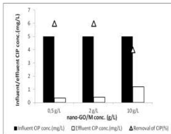
**Figure 1d:** Comparison of increasing concentration of nano-GO/M (0.5, 2 and 10 g/L) on the yields of CIP removal for constant CIP concentration (5 mg/L) at pH=6.5, at 21°C and 30 min contacting time
