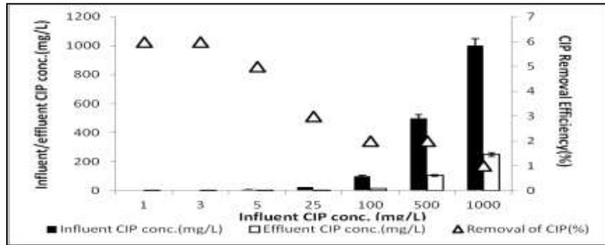
**Figure 3:** Effect of increasing CIP concentration on the yields of CIP removal at a nano-GO/M concentration of 0.5 g/L at pH=6.5, at 21°C and 30 min contacting time
