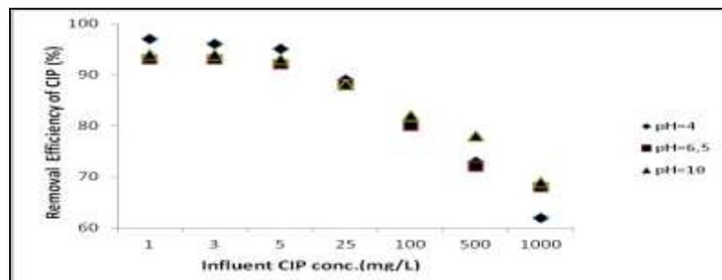
**Figure 8:** Effect of different pHs (4, 6.5 and 10) on the yield of CIP removal at a nano-GO/M concentration of 0.5 g/L at pH=6.5, at 21°C and 30 min irradiation time
