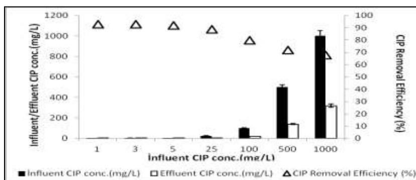
**Figure 9:** Effect of increasing CIP concentrations (1 mg/L, 3 mg/L, 5 mg/L, 25 mg/L, 100 mg/L, 500 mg/L, 1000 mg/L) on the yield of CIP removal at a nano-GO/M concentration of 0.5 g/L at pH=6.5, at 21°C and 30 min irradiation time
