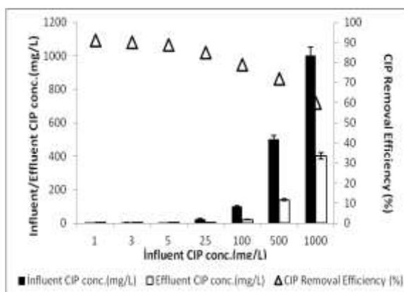
**Figure 6c:** Effect of increasing CIP concentration on the yields of CIP removal at a nano-GO/M concentration of 10 g/L at pH=6.5, at 21°C and 30 min contacting time by photooxidation.
