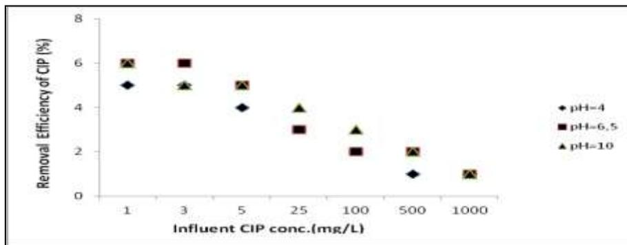
**Figure 4:** Effect of different pHs (4, 6.5 and 10) on the yield of CIP removal at a nano-GO/M concentration of 0.5 g/L at pH=6.5, at 21°C and 30 min contacting time
