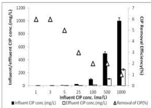
**Figure 1a:** Effect of increasing CIP concentration on the yields of CIP removal at a nano-GO/M concentration of 0.5 g/L at pH=6.5, at 21°C and 30 min contacting time
