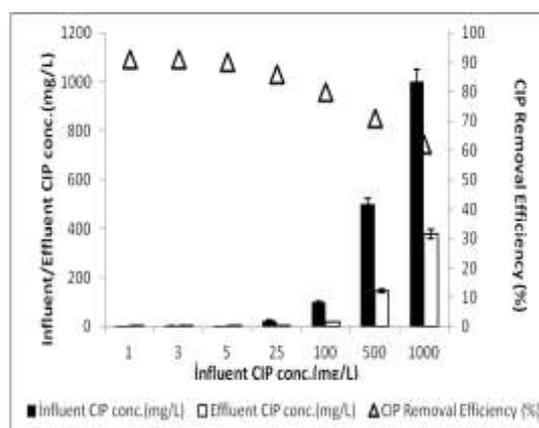
**Figure 6b:** Effect of increasing CIP concentration on the yields of CIP removal at a nano-GO/M concentration of 2 g/L at pH=6.5, at 21°C and 30 min contacting time by photooxidation.
