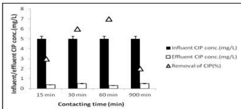
**Figure 2:** Effect of contacting time on the yields of constant CIP concentration (5 mg/L), at a constant nano GO/M concentration (0,5 g/L), at a pH of 6.5 and at 21°C
