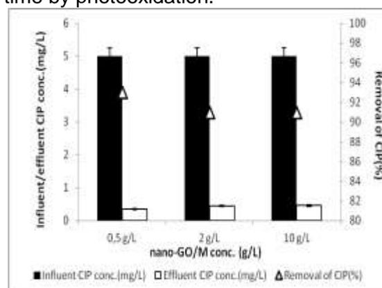
**Figure 6d:** Comparison of increasing concentration of nano-GO/M (0.5, 2 and 10 g/L) on the yield of CIP removal for constant CIP concentration (5 mg/L) at pH=6.5, at 21°C and 30 min contacting time by photooxidation.
