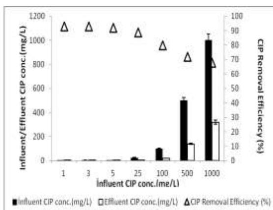
**Figure 6a:** Effect of increasing CIP concentration on the yields of CIP removal at a nano-GO/M concentration of 0.5 g/L at pH=6.5, at 21°C and 30 min contacting time by photooxidation
