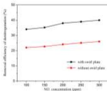
**Figure 3.** Influence of the swirl plate on separate denitrogenation (gas velocity: 1.5 m/s, liquid-gas ratio: 14.3 m<sup>3</sup>/L)
