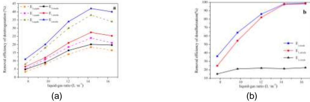
**Figure 5:** Influence of liquid-gas ratio on removal efficiency (superficial velocity: 1.5 m/s, NO<sub>x</sub> concentration: 200 ppm, SO<sub>2</sub> concentration: 1000 ppm)
