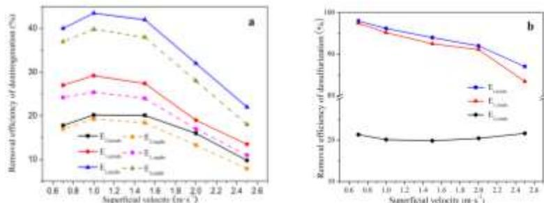
**Figure 4.** Influence of superficial velocity on removal efficiency (liquid holdup 9.7 m<sup>3</sup>/h, NO<sub>x</sub> concentration: 200 ppm, SO<sub>2</sub> concentration: 1000 ppm)
