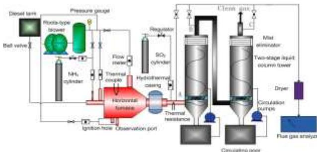
**Figure 1:** The schematic of the simultaneous desulfurization and denitrogenation system
