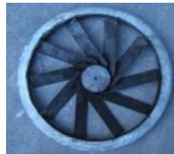
**Figure 2:** The schematic of the swirl plate in liquid column tower
