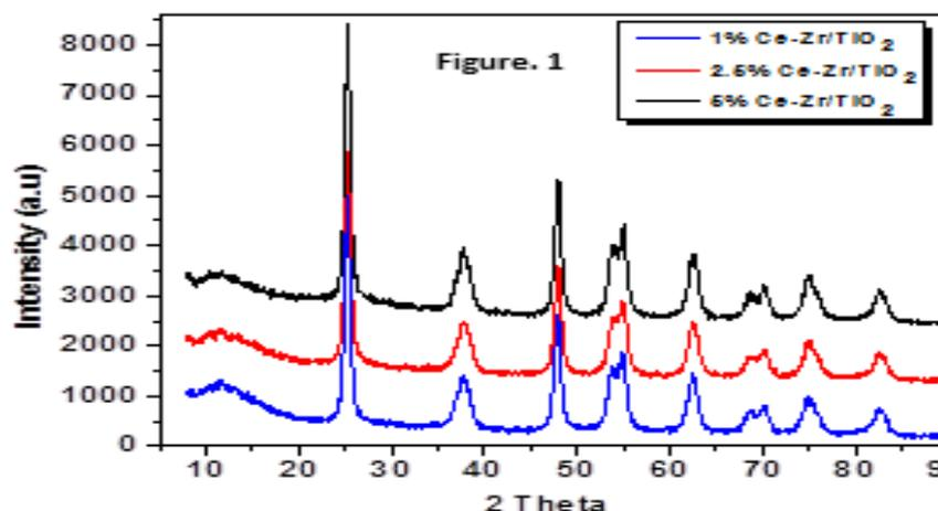
Figure 1: XRD spectra 1%, 2.5% & 5% Ce-Zr loaded on TiO<sub>2</sub> catalyst
