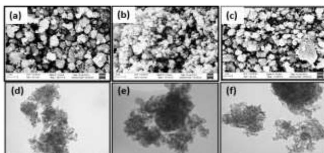
**Figure 3:** SEM images (a, b, c) and TEM images (d, e, f) of 1%, 2.5% & 5% Ce-Zr on TiO<sub>2</sub>
