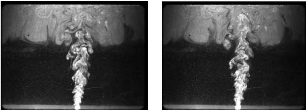
**Figure 2:** Photographs of a buoyant jet (differed by 0.25 s).
