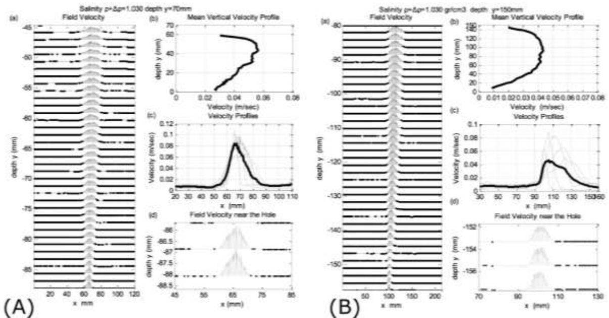
**Figure 4:** Buoyant jet with  $\rho_0=1.000$  gr/cm<sup>3</sup>, salt water with  $\rho_a=\rho+\Delta\rho=1.030$  gr/cm<sup>3</sup> and water depth: (A)  $y=70$  mm, and (B)  $y=150$  mm.
