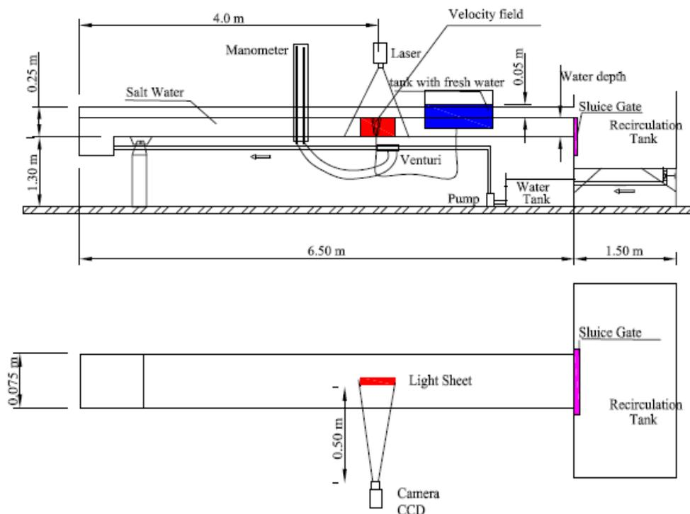
**Figure 1:** Experimental set-up (open channel).
