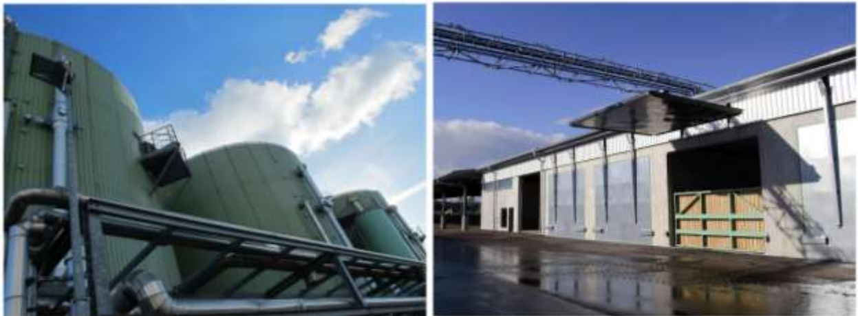
Figure 2: An example of a continuous wet reactor (on the left) and a batch dry battery of reactors (on the right).
