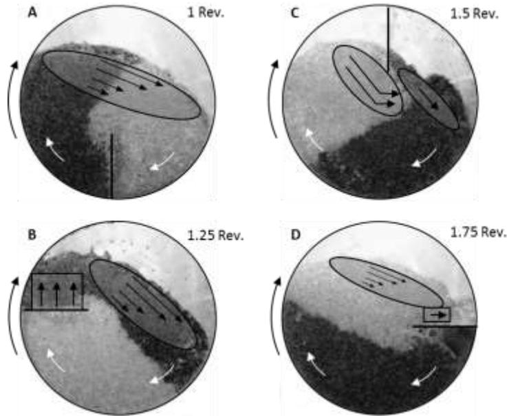
**Figure 2:** Flow patterns for substrate 1 inside the RDF (fill level: 0.80) influenced by a baffle ( $L = 0.16$  m).
