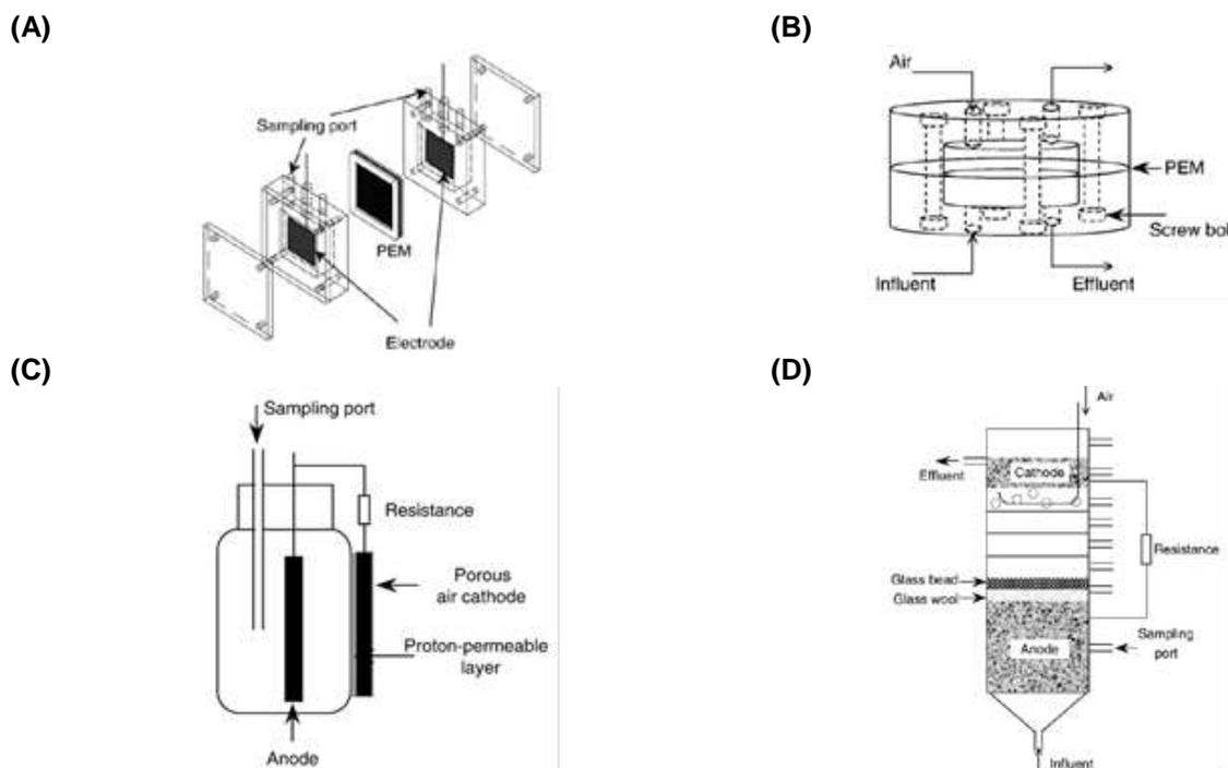
**Figure 1:** Schematic representation of different MFC configurations (A) cube type dual chamber MFC (B) miniature MFC (C) single chamber air cathode MFC and (D) upflow MFC (Du *et al*, 2007)
