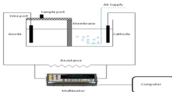
**Figure 2:** Schematic representation of MFC set-up
