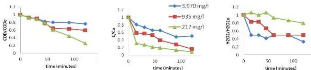
**Figure 2:**  $H_2O_2/O_3$  treatment of distillery wastewater at varying initial wastewater concentration (initial  $H_2O_2$  concentration: 500 mg/L;  $H_2O_2/O_3 = 0.8$ ; without initial pH adjustment): Significant differences for both Color and  $H_2O_2$  consumption plot ( $p < 0.05$ ), none for COD.
