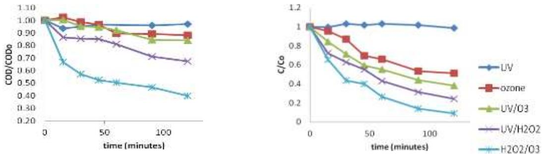
**Figure 3:** COD and color profile of various advanced oxidation treatment of distillery wastewater (initial COD ~1000 mg/L; initial H<sub>2</sub>O<sub>2</sub> concentration ~1,000 mg/L; without initial pH adjustment)
