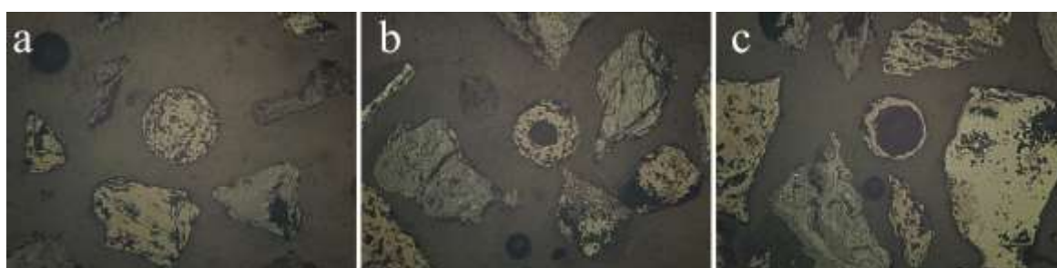
Figure 3: Optical microscopy images of magnetic particles from thin polished sections of magnetic extracts from road dusts.
