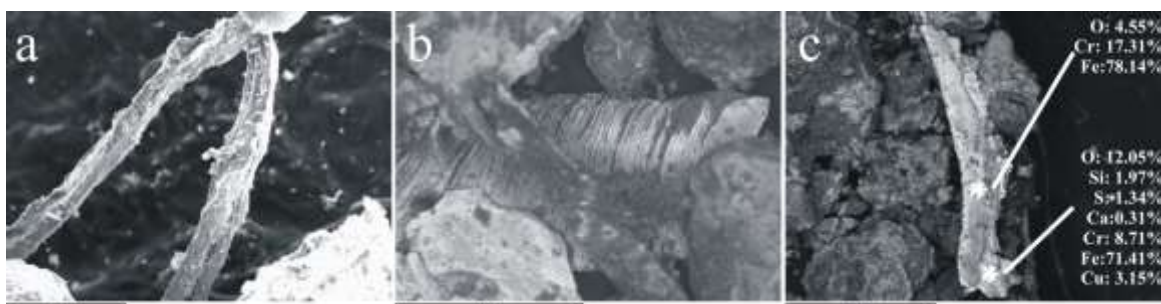
Figure 2: Backscattered SEM images of angular magnetic particles.
