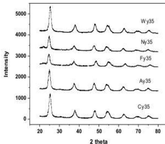
**Figure 2:** XRD spectra of synthesized photocatalysts doped with individual dopant precursor
