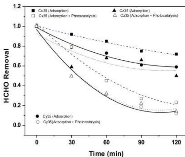
**Figure 5:** Residual formaldehyde plot using synthesized photocatalysts with varying dopant molar concentrations. 0.1 g/L photocatalyst, 2ppm formaldehyde, 30 0C, Adsorption (0 W/m<sup>2</sup>), Photocatalysis (Vertical 10W/m<sup>2</sup> / Horizontal 25W/m<sup>2</sup>).
