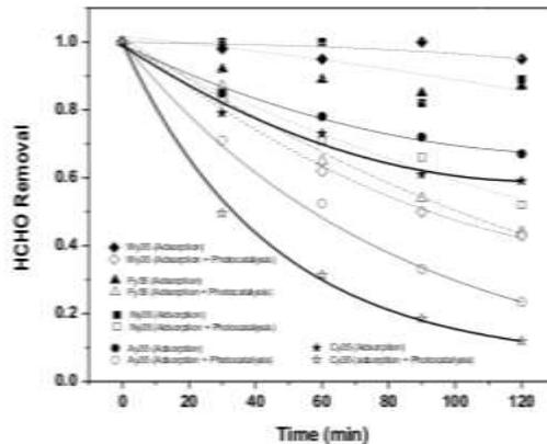
**Figure 1:** Effect of individual dopant precursor on photocatalytic rate. Experimental Conditions: 0.1g/L catalyst, 2ppm initial formaldehyde concentration, 30C, 25.7 W/m<sup>2</sup>
