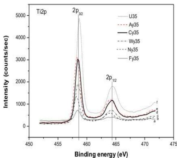
**Figure 4:** Ti2p XPS spectra of the different dopant used in the synthesized photocatalyst, a. Fy35, b. Ny35, c. Wy35, d.Cy35, e.Ay35, f. U35
