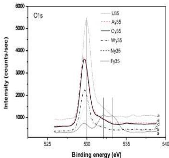
**Figure 3:** O1s XPS spectra of the different dopant used in the synthesized photocatalyst, a. Fy35, b.Ny35, c. Wy35, d.Cy35 e. Ay35, f. U35
