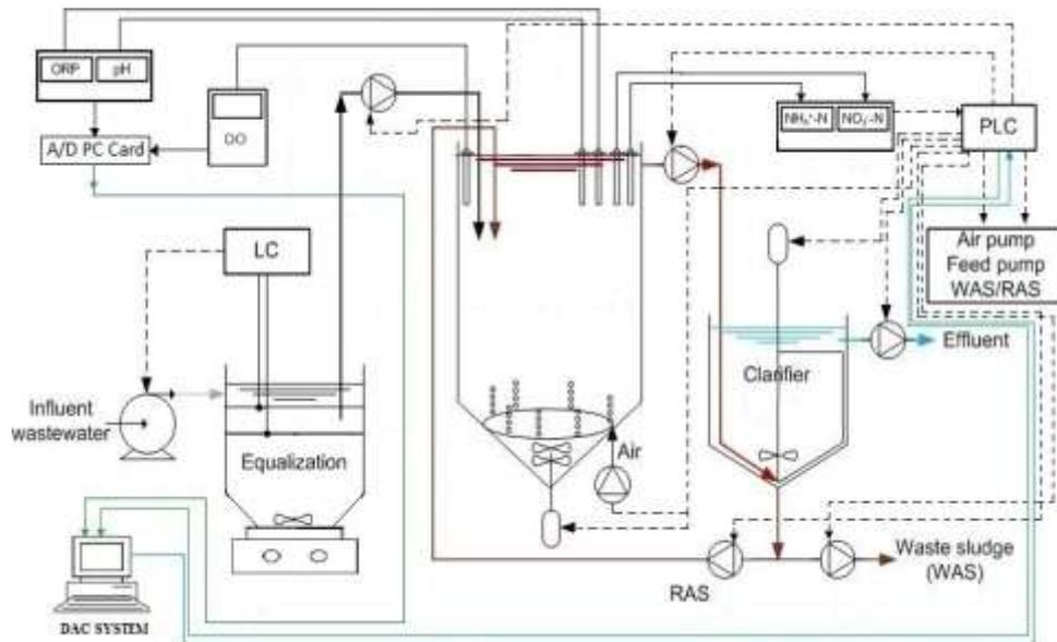
**Figure 1:** Schematic layout of an intermittently aerated and fed activated sludge pilot plant.
