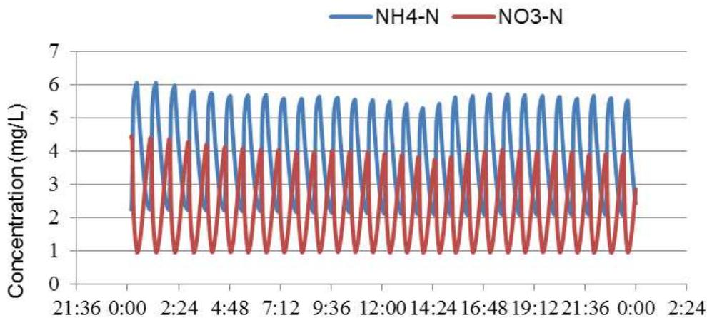
**Figure 2:** NH<sub>4</sub>-N and NO<sub>3</sub>-N cycle profiles during monitoring of the nitrification-denitrification process in intermittently aerated and fed bio-reactor.
