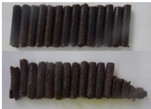
Figure 7: Pellets produced with particle size 0.5-0.25 mm, temperature 92 °C, moisture content w.b. 10.6 % (top) 20.2 % (bottom).
