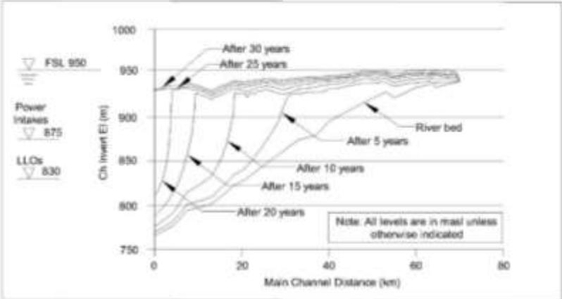
**Figure 1:** Sediment profile by maintaining RWL at FWL (no flushing).
