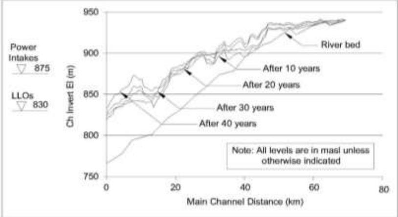
**Figure 2:** Sediment profile under free flow flushing.
